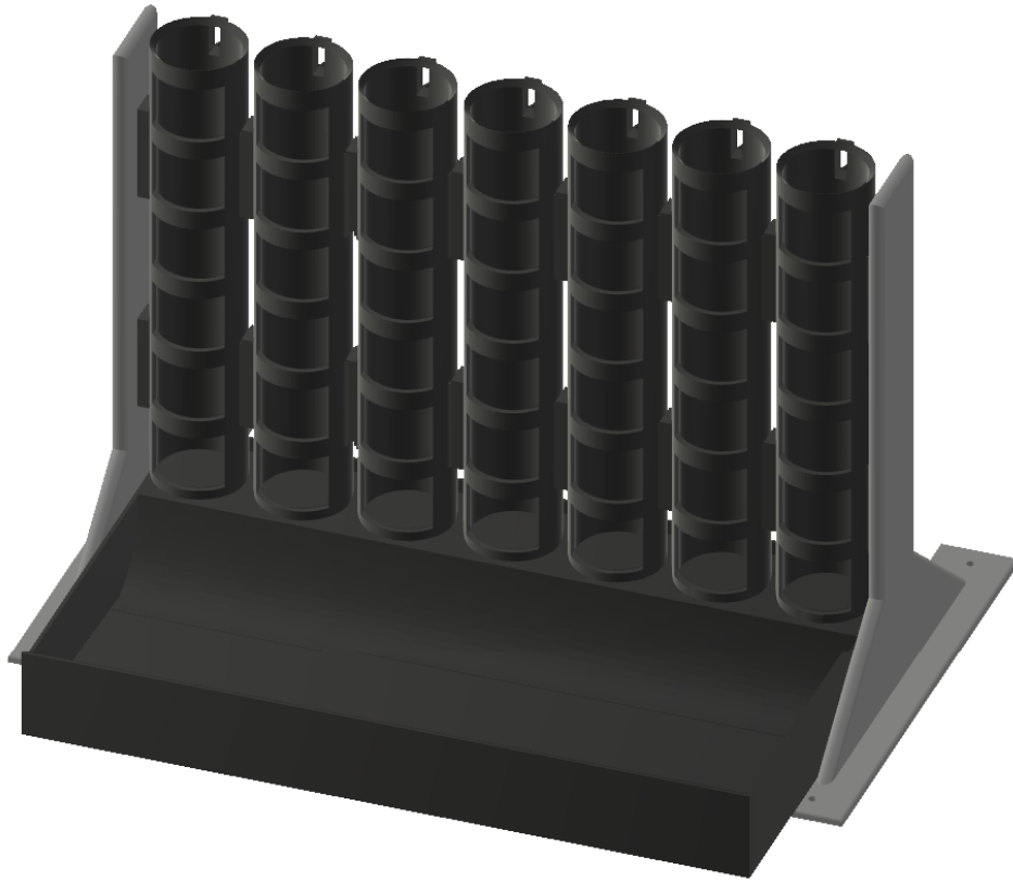
Figure 5.6 | Assembled game board for Connect Four. Seven tubes, two stands and a tank build together the game board. The tubes and the stands are connected with t-profiled guide rails. The tank is placed below the tubes.
